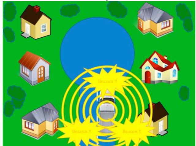
Figure 1: The first implementation requires a vehicle to be within transmission range of each house to receive meter data
